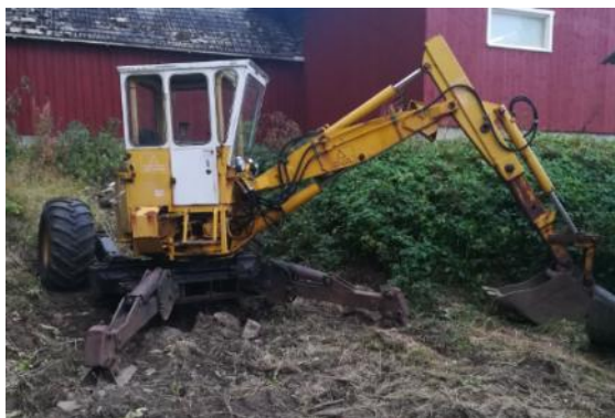
Menzi Muck gravemaskin
