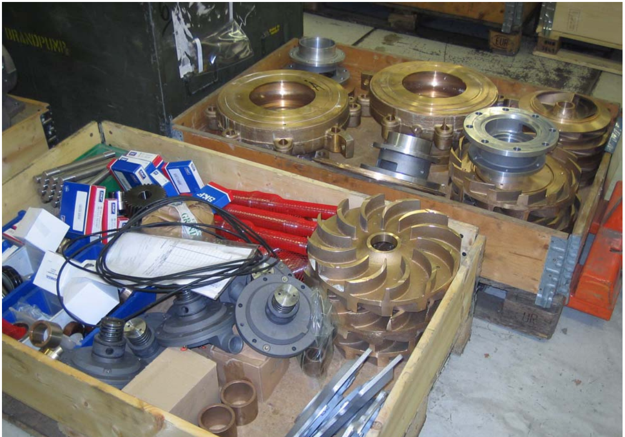
Pumpedeler klar for montering
