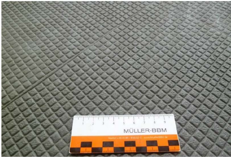
Figure 5 – small scale test of low noise surface in UHPC
