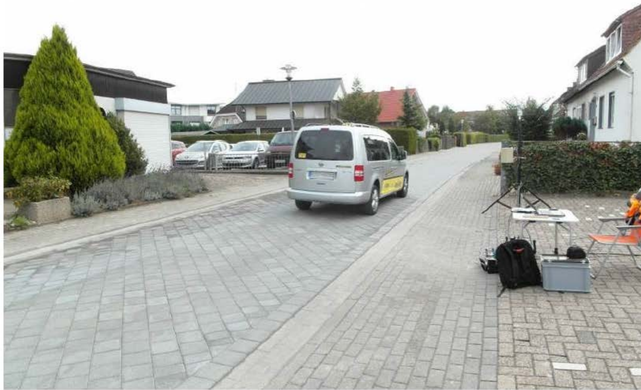
Figure 12 – Test track of porous concrete block pavement during SPB measurements
